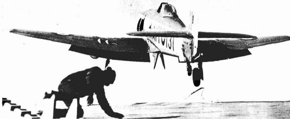
A Sea Fury hurtles from the deck of the "Magnificent" during Exercise Mariner and, almost before the aircraft is airborne, an engineer mechanic scrambles from his sponson to retrieve the catapult stop for the next plane. (MAG-4981)
