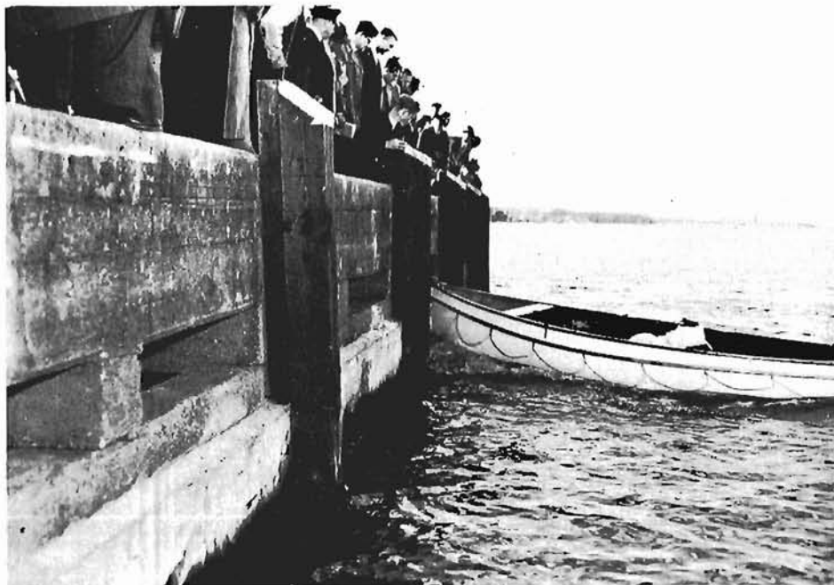
Crouched low to avoid going overboard, Lieut. (E) R. G. Guy drives a Canadian-built fibreglas dinghy at a ten-knot clip against the concrete town wharf at Arnprior, Ont. He later rammed it aground on the rocky shoreline. In neither case was any damage done. (O-6008)
