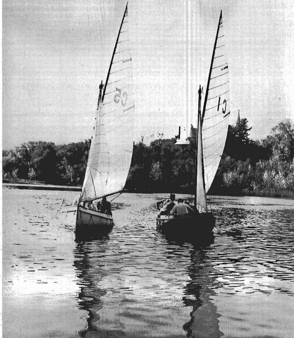
Crews compare the performances of two dinghies under sail. On the left is a prototype 14-foot dinghy built of polyester resin reinforced with fibreglas cloth and mats. It is the first boat of this type of construction to be built for the RCN. (O-6014)
