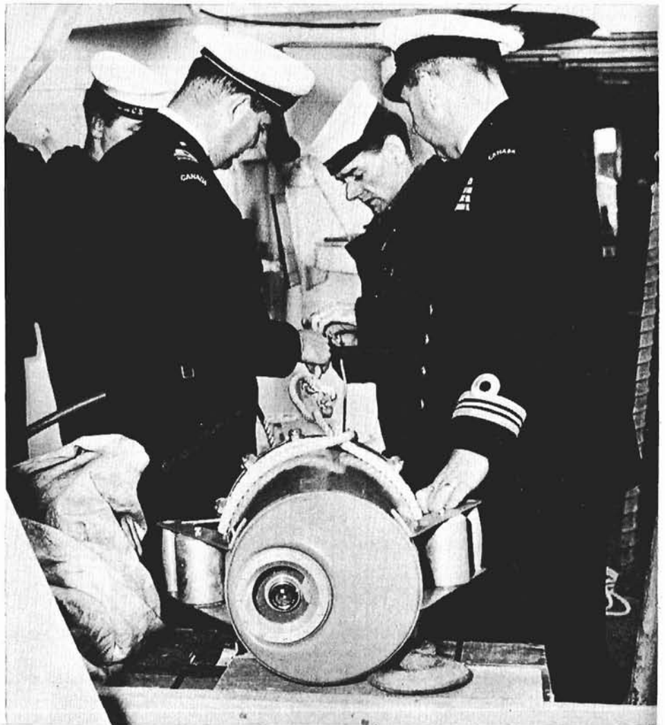
The eye that sees below the sea, the underwater television camera carried in HMCS Labrador is prepared for lowering into Halifax harbour during tests carried out there before the Arctic patrol vessel sailed for the north. Lt.-Cdr. Jack Bathurst, of Ottawa, (right), underwater TV expert, instructed Labrador crew members in the use of the equipment, which will be used to survey the approaches to Arctic shorelines. Lt.-Cdr. John Ruse and PO William McPhee attach a security line to a strop before lowering away. (LAB-686)
