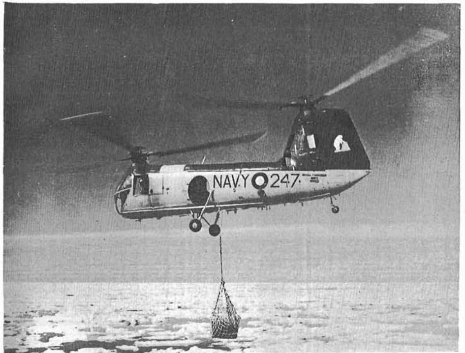
The Piasecki helicopter borne in the Labrador carries a drum of oil ashore to an electronic position indicator station. Two smaller Bell helicopters are also attached to the Arctic patrol ship. (LAB-960)
