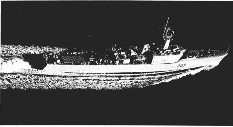
The new anti-submarine destroyer escorts of the Royal Canadian Navy are designed to operate away from base facilities for as long as two months—nearly twice the length of time a Second World War destroyer could go without dockyard attention. With shore bases knocked out in an atomic war, the ability of warships to continue the fight at sea might spell the difference between defeat and victory, according to some military experts.
