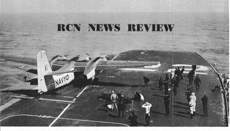
A Tracker anti-submarine aircraft surges forward on the steam catapult of the Bonaventure during flight trials this spring in United Kingdom waters. (BN-608)
