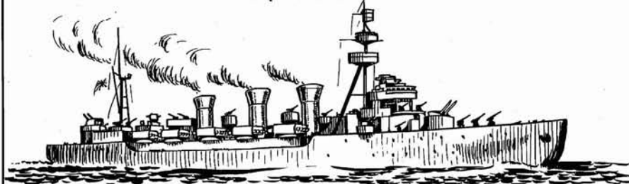
JAPANESE 'KUMA' CLASS CRUISERS, REFITTED AS 'TORPEDO CRUISERS' IN WORLD WAR II, CARRIED THE HEAVIEST TORPEDO ARMAMENTS AFLOAT... FORTY 24-INCH TORPEDO TUBES.
