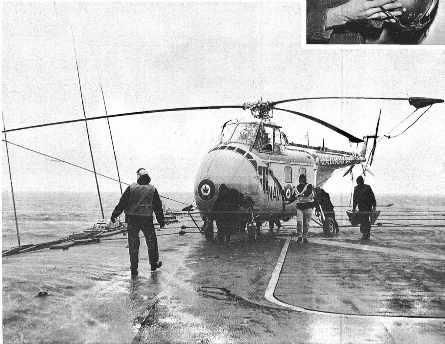
Spray swept from the grey sea by the Arctic wind forms rivulets on the Bonaventure's flight deck as "Pedro", the rescue and utility helicopter is repositioned. The flexible rotor blades are lashed down to keep the motion of the ship from snapping them. The picture was taken during Exercise Traplaine. (HS-66400-108)
