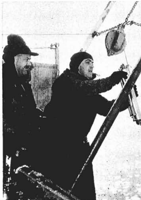
Both temperature and salinity have profound effects on the transmission of sonar beams in the sea. Here a scientist samples the salinity of the Gulf of St. Lawrence by means of metal bottles which can be set to admit water at any chosen depth. (LAB-1475)
