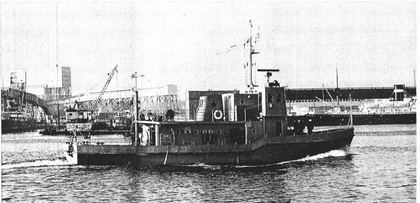
A custom-built diving vessel, YMT-11, was completed in January at Ferguson Industries, Pictou, N.S., for the Navy and began trials off Halifax. She is 88' by 20' by 4'9", with a speed of nearly 11 knots, can dive four men at a time to about 250 feet and is fitted with a recompression chamber. (HS-67277)
