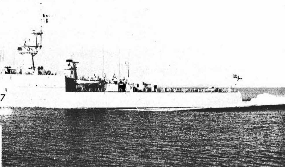
Light, tough and weather-resistant are the plastic gun shields developed by the RCN to protect the intricate mechanisms of the 3-inch-50 guns in the destroyer escorts. The shields are visible both fore and aft in this picture of HMCS Skeena. (E-60468)
