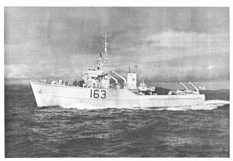
HMCS Miramichi, is one of the RCN's postwar Bay class minesweepers. These wooden sweepers are equipped to deal with a variety of mines. (E-43508)
