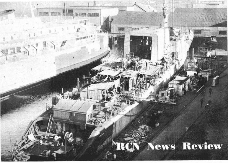
Here is a visual progress report on the transformation of HMCS Assiniboine. Her stern has already been remodelled to accommodate variable depth sonar and construction of the helicopter hangar is well advanced. (E-70700)
