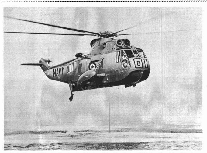
The first Sikorsky CHSS-2 twin-turbine all-weather helicopters will be delivered to the RCN in May. Nine of these helicopters are being obtained during the 1963-64 fiscal year. Each will carry a crew of four, two pilots and two sonar operators. Equipped with the latest navigation, detection and weapon systems, the CHSS-2 will be capable of locating, tracking and attacking a submarine while operating in conjunction with or independently of surface ships. (CN-6572)
