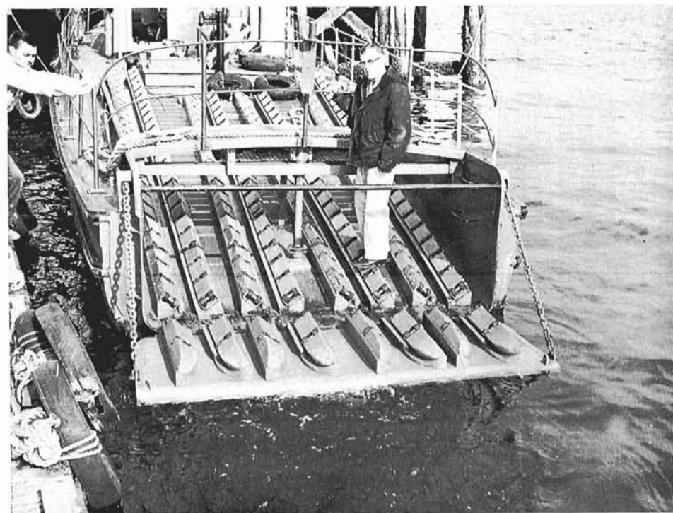
The little CNAV Wildwood, based at Esquimalt, has become a somewhat specialized craft and her appearance could well be a puzzler to anyone not familiar with her task of recovering torpedoes after practice runs. Her roller-equipped ramps simplify the task of taking spent torpedoes from the sea. (E-72172; E-72173)
