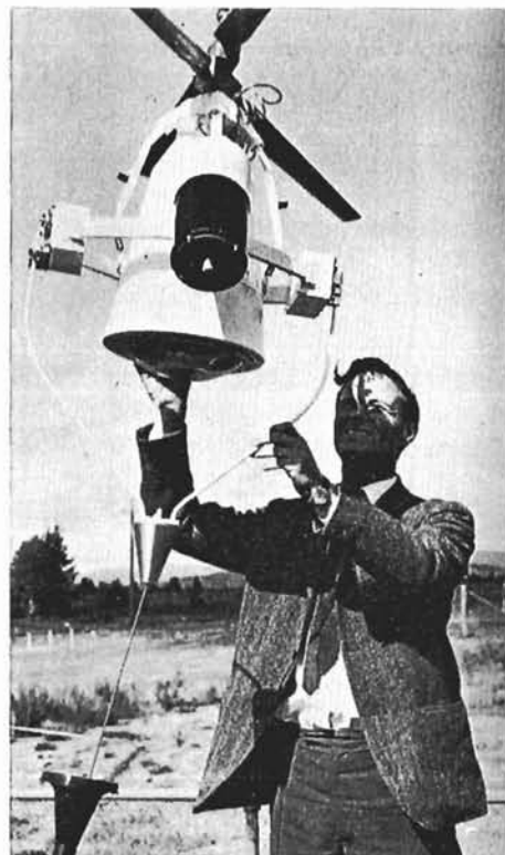
Project engineer, Christopher Wilson, of the Canadian Armament Research and Development Establishments, Valcartier, Que., demonstrates the lightness of the airborne components of the periscope, a DRB-designed surveillance device. A winch on the control vehicle stores the tethering cable and permits raising and lowering of the airborne components. (DRB Photo)
