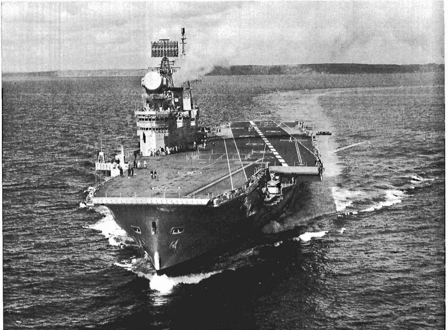
After a major reconstruction that took nearly five years, HMS Eagle is at sea again as Britain's most up-to-date aircraft carrier. The greatest outward change is the addition to the island of the 984 radar scanner. Down below tremendous changes have been made, including the installation of an inertial navigation system, ordinarily fitted only in submarines. (Photo courtesy British Information Services)
